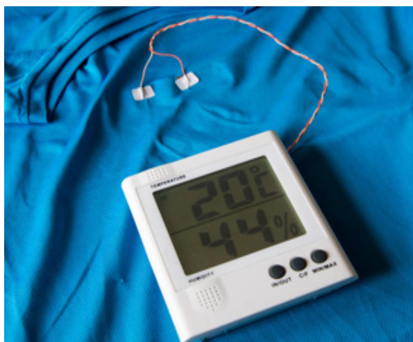
Figure 12. Digital thermometer/hygrometer sensor and LED lightning system powered by textile SCs produced by WEStoreOnTEX.
