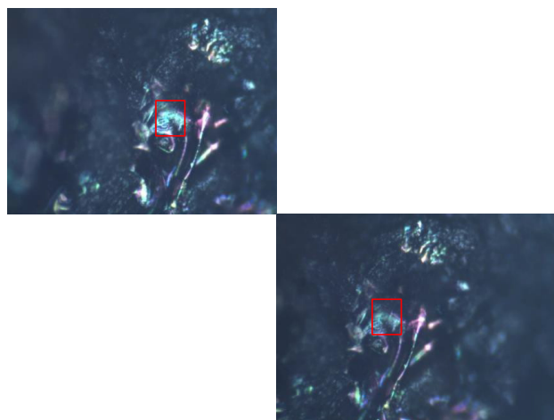
Figure 4. Optical image of the carbon foam showing an overall view of the porous structure of the foam. The squares show the areas of the carbon foam where the Raman spectra were obtained.
