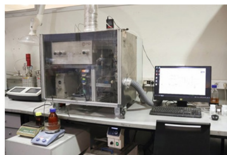
Figure 1. Schematic representation and laboratory set-up of the continuous trickle-bed reactor used for HDO experiments.
