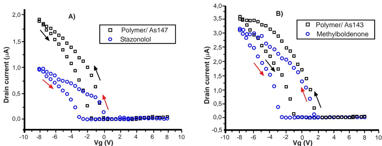
**Figure 6.**  $I_{DS}/V_G$  plots of typical CNTFETs. (A) After anchoring the polymer and As147 antibody (black) specific for Stz and after anchoring stanzonolol (blue). (B) After anchoring the polymer and As143 antibody (black) specific for MB and after anchoring methylboldenone (blue).
