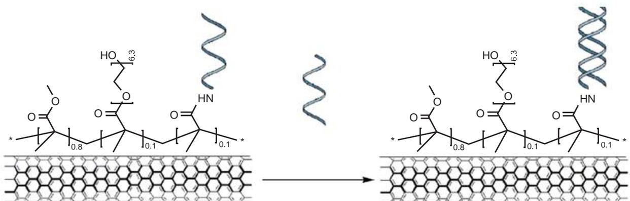
**Figure 4.** Schematic representation of the DNA hybridization after bonding the aminated DNA single sequence to the polymer in the CNTFET.
