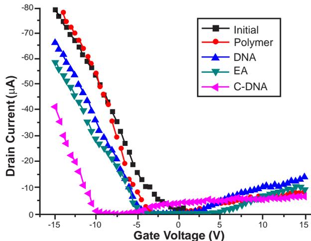
**Figure 5.**  $I_{DS}/V_G$  plots of a typical device for the direct swept of: the bare device, after anchoring the polymer, after simple sequence DNA bonding, after blocking the succinimidyl groups with EA and in the hybridization step with the complementary sequence.
