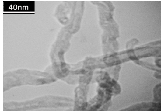
Figure 1. TEM micrograph obtained from raw CNTs.
