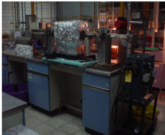
Figure 1(b) Pyrolysis reactor to produce activated carbon from Pecan nut shell.
