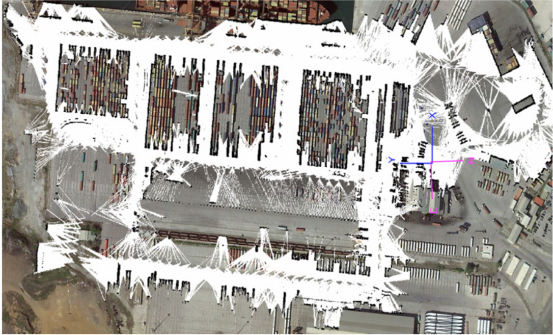
Figure 11. The map is overlaid onto a georeferenced image using the optimized EN-to-SLAM frame transformation (X,Y,\theta)=(4.01m, 3.42m, 3.177rad) with an EN origin at (lat,lon)=(40.638972,22.907978) . Notice that the image and the map correspond to different days and hence some of the mapped features do not match.
