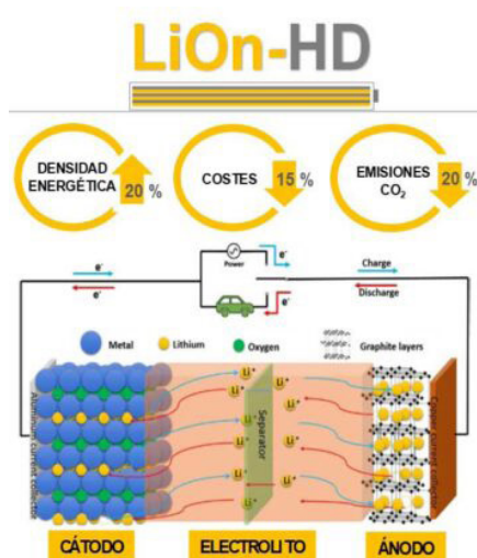
Image: Pictorial representation of project LiOn-HD. The target improvements over conventional Li-ion batteries is shown on the left: 20% increase of energy density, 15% cost reduction, and 20% reduction of CO 2 emissions.
