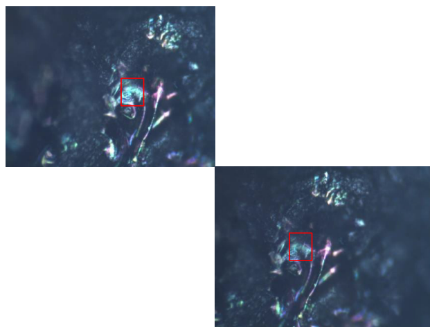
Figure 4. Optical image of the carbon foam showing an overall view of the porous structure of the foam. The squares show the areas of the carbon foam where the Raman spectra were obtained.
