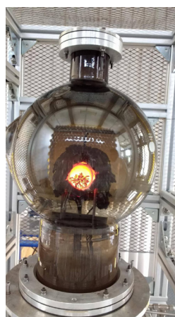
Figure 1. a) Photograph of the solar reactor and b) sketch of the concentrated solar technology "solar furnace" and reactor.
