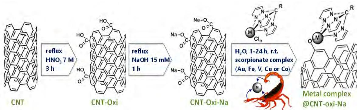
**Figure 3:** Immobilization of C-scorpionate complexes onto carbon nanotubes (R = H; CH<sub>2</sub>OH).
